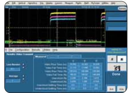
▶ RGB Transient Response Measurement Results (Option VGA).
